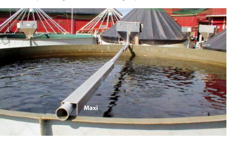
The feeder utilizes a screw mechanism for distributing feed and can be customized to fit most tanks and walkway solutions. Independent tests have shown that spreading the feed throughout the tank leads to better growth and less fin erosion.
