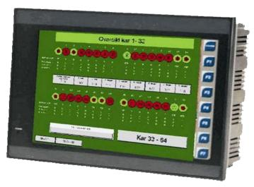
Automatic feeding for up to 96 feeders. In cooperation with Norwegian smolt farmers, Betten has developed a highly user-friendly PLC system, featuring overview or detailed images for each individual tank.
